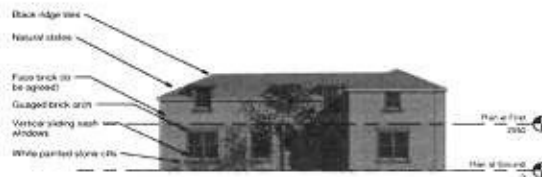
④ Elevation towards courtyard 1 : 100
